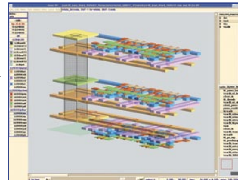
Actual screenshot of MAX-3D Layout Editor – True Through-Silicon Via (TSV) layout and editing using multiple technologies at the same time.
