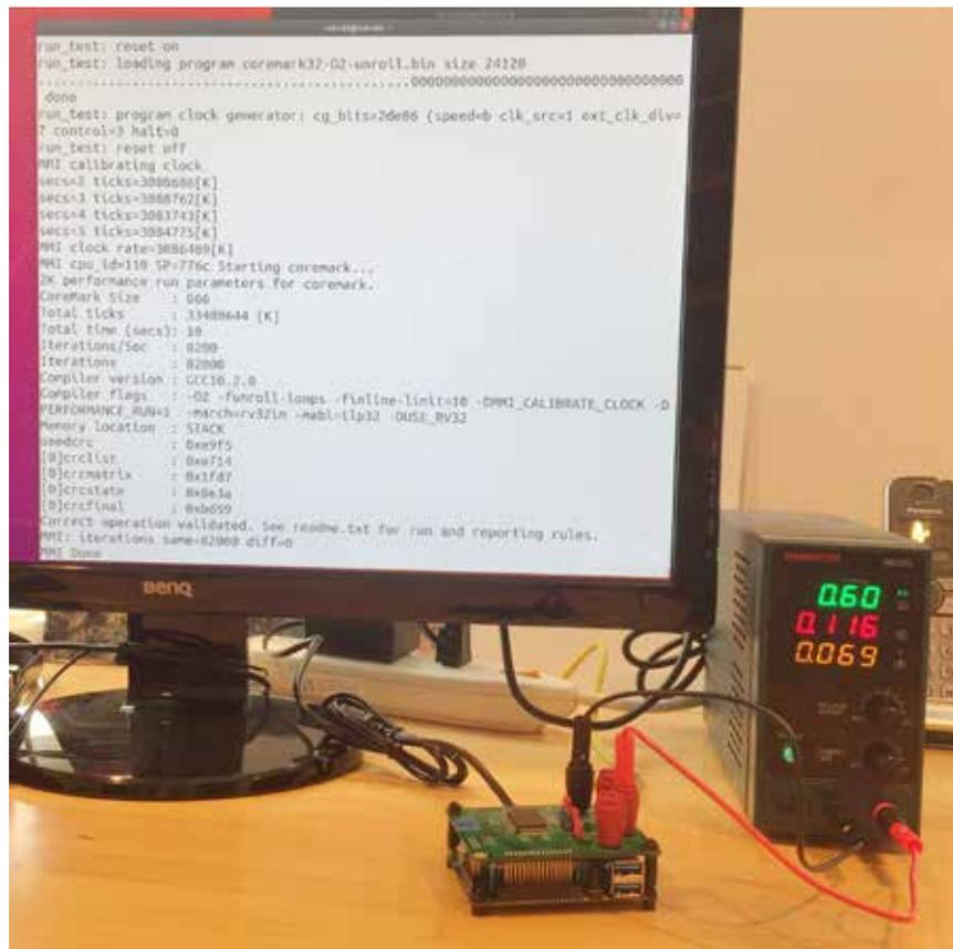
**Micro Magic RISC-V demo on Odroid board showing 110,000 CoreMarks/Watt**
